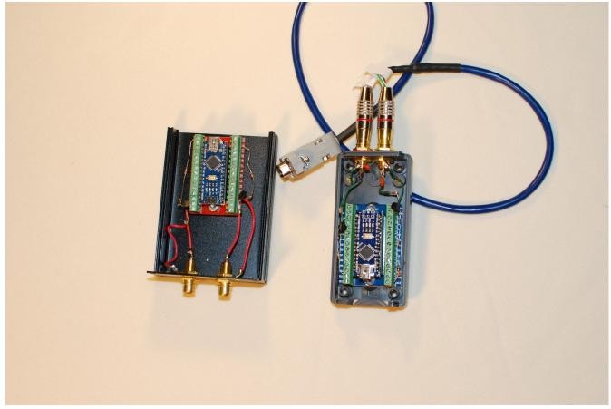
A cable needs to be made for your radio: two male RCA plugs to the TinyFSK, and an appropriate end
