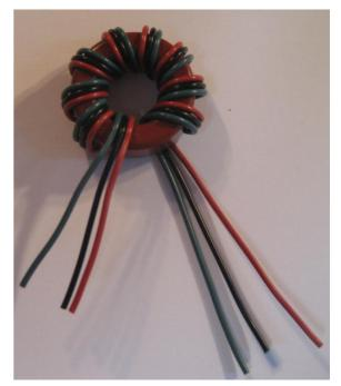
Next, trim, crimp together and solder <u>the left black wire</u> with the <u>right red wire</u> When the step is completed, it will look like the photo on the right:
