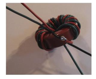
The next three steps should appear as shown in the right photo. Crimp and solder a #10 lug to the *left red* wire about 2" from the toroid. The completed lug will later connect to the antenna connection bolt on the top side of the enclosure.
